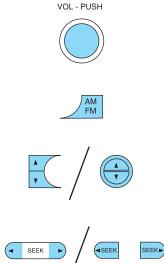
Press ◀ SEEK ► to search down/up the chosen frequency band for the next strongest station. To disengage SEEK mode,
